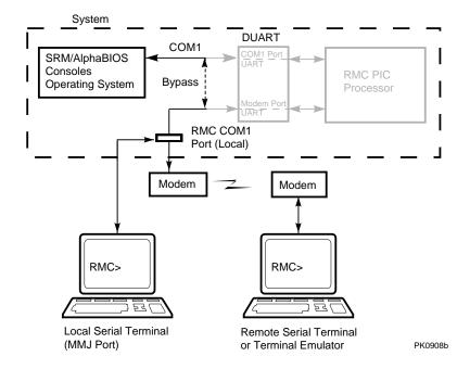
**NOTE:** The internal system COM1 port should not be confused with the external COM1 serial port on the back of the system. The internal COM1 port is used by software to send data either to the COM1 port on the system or to the RMC modem port if a modem is connected.
