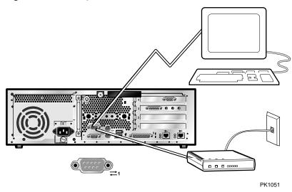
You can connect a terminal or a modem to the COM1 port, but not both at the same time. You use the terminal to set RMC parameters for the connection, then connect the modem. See Section 4.9.
