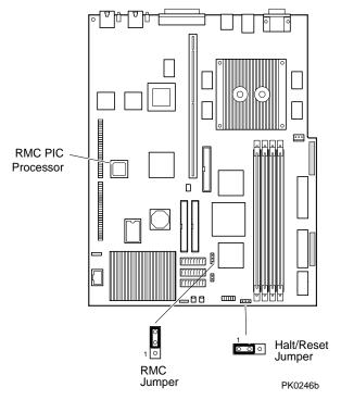
The RMC logic is implemented using an 8-bit microprocessor, PIC17C44, as the primary control device. The RMC PIC is programmed with code to control access to various environmental status bits.
